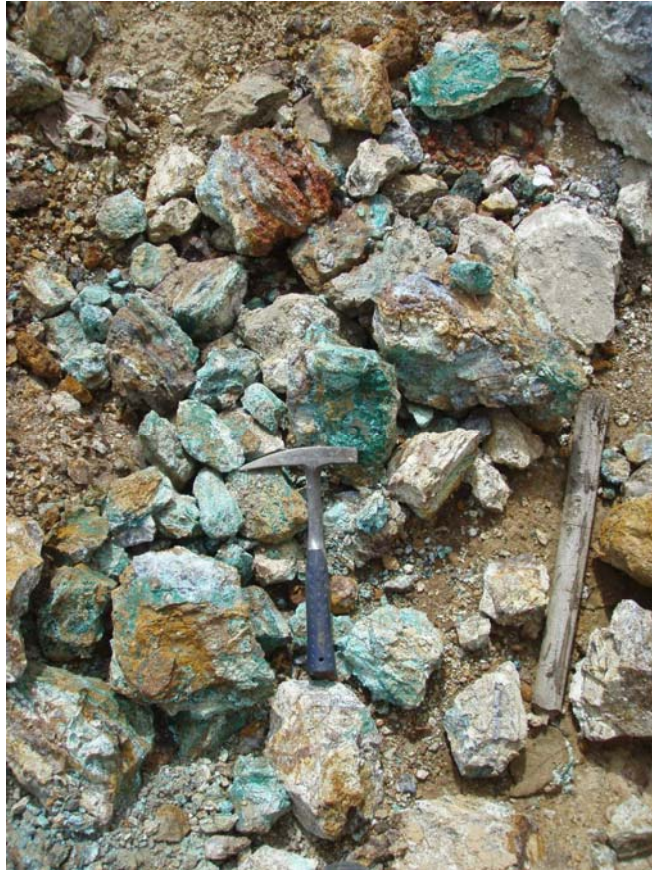
Photograph of copper stained and gold mineralised rocks excavated by hand in the Nam Thong mining lease.
