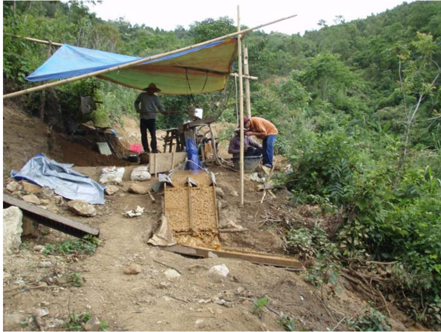
Artisanal miners at the Nam Thong mining lease using a sluice box to concentrate gold particles from soil and crushed bedrock.
