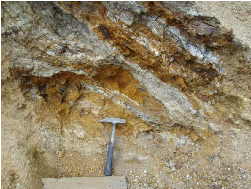
Photograph of iron and copper stained outcrop of gold mineralised siltstone in the Nam Thong mining lease.
