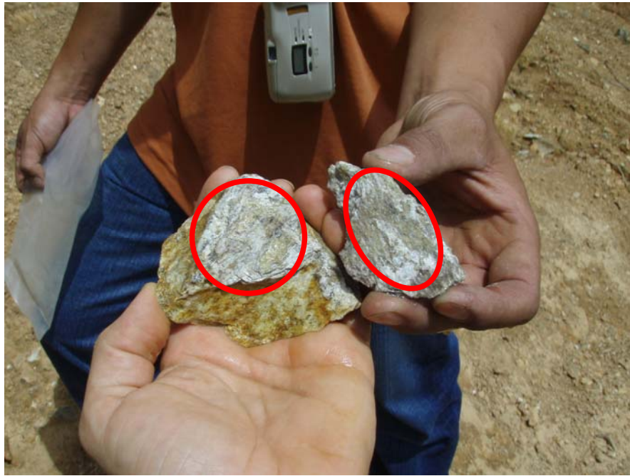
Photograph of sheared limestone specimens containing visible gold from the Nam Thong mining lease.
